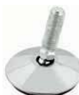
art.405 pag.21 piedino regolabile in pa - ghiera cromata perno fe zincocromato snodato chiave 10 levelling element in pa chrome plated ferrule and zinc-plated steel joint stud mm 10
