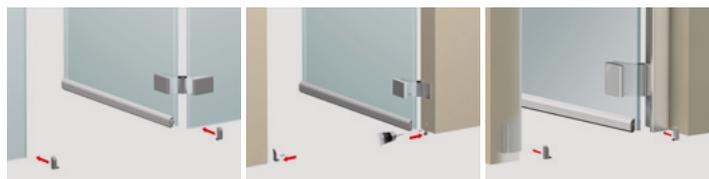
Mechanism with a single adjustment (screw F: descent) characterised by the controlled movement of the moving profile with gasket (immediate descent from the hinge side of the door and consequent gradual descent for the entire length) for adjustment to the floor.
