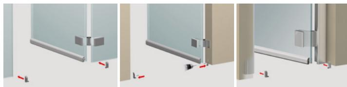
Extruded profiles in aluminium alloy 6060 - anodized or painted, extruded tubular EPDM gasket - elements printed in self-lubricating nylon + nylon reinforced with 30% glass fibre - threaded rods in burnished iron - Ø 5 mm brass bushing and Ø 6 mm brass bushing - coil springs in treated stainless steel.
